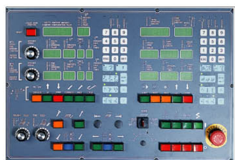
The control panel integrated with NC wheel dressing device
